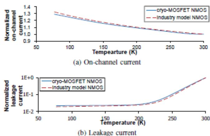
Figure 2.2. From [2.1], MOSFET  $I_{on}$  and  $I_{off}$  versus temperature.
