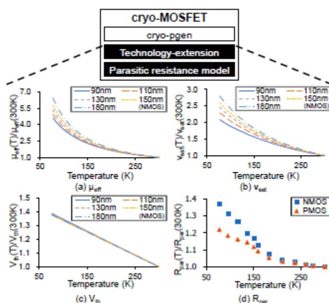
Figure 2.1. From [2.1], Extension to the baseline MOSFET model: (a) Carrier mobility; (b) Saturation velocity; (c) Threshold voltage; (d) Parasitic resistance model.
