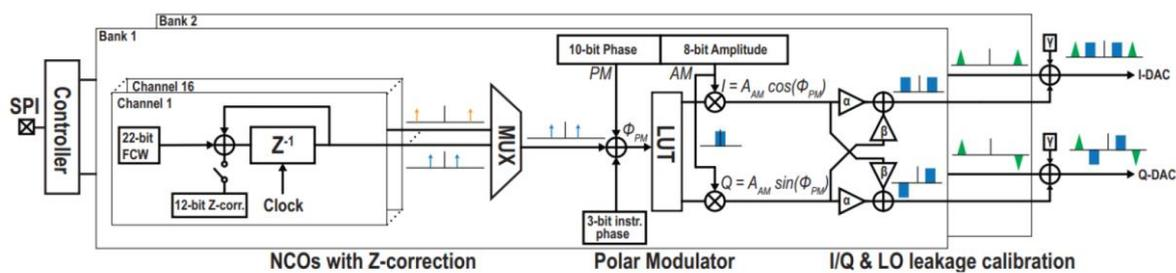
Figure 3.1. Intel approach, the circuit is in FFT 22nm and works at 4K.
